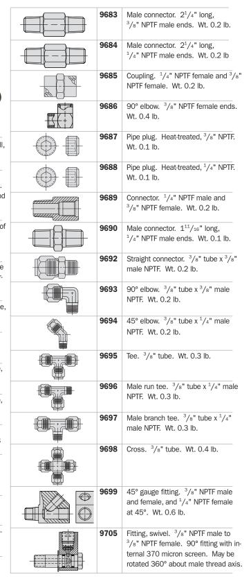
NOTE: Power Team hydraulic fittings are intended for use with our high pressure hydraulic products and are suitable for use at max. working pressures of 10,000 psi unless otherwise noted.
